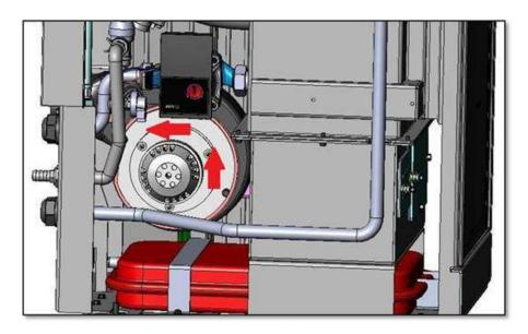
2a) Open the door of the boiler and open the inspection cap as show in the picture below;
